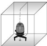
Front vertical and plumb point
